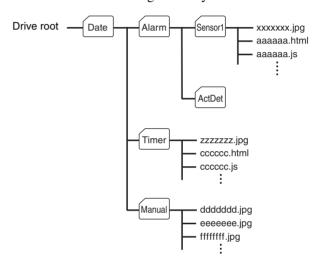
A \_\_\_\_\_ represents a folder created automatically. The Date folder has a 6-digit folder name consisting of the lower two digits of year (2 digits), month (2 digits) and date (2 digits). The Sensor, and Act Det (activity detection) folders correspond to alarm modes. The Timer folder corresponds to the periodical recording mode. And, the Manual folder corresponds to the manual mode.
